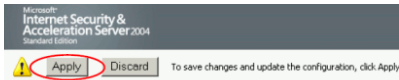
Figure D.4. ISA Server 2004/2006 - Applying changed log settings
